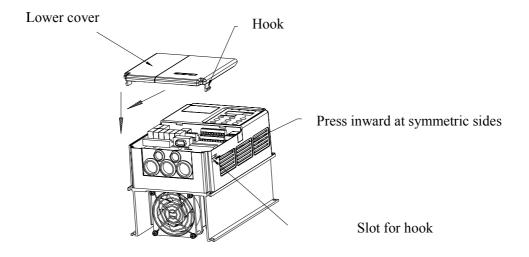
Fig.3-2 Remove the bottom cover
