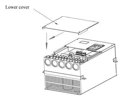
Fig.3-3 Remove the metal bottom cover
