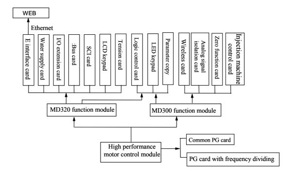
Fig.2 Architecture of MD series inverter
