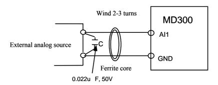
Fig. 3 -7 Analog Input Terminal With Filter devices
