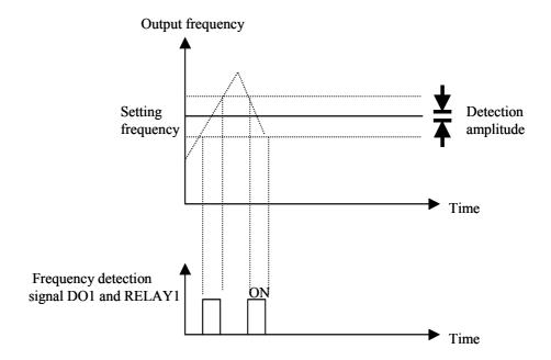
Fig. 6-7 Frequency Reaching Checkout Amplitude Value
