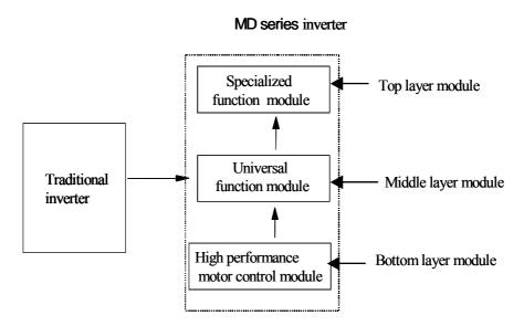
Fig. 1 Comparison between traditional inverter and MD series inverter
