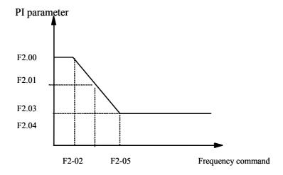
Fig. 6-2 PI Parameters Schematic Diagram
