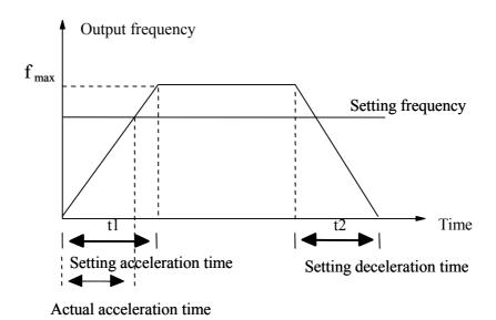
Fig. 6-1 Acceleration/Deceleration Time Schematic Diagram
