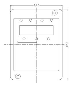
Fig.2-3 Keypad Appearance and Dimension of Installation Holes
