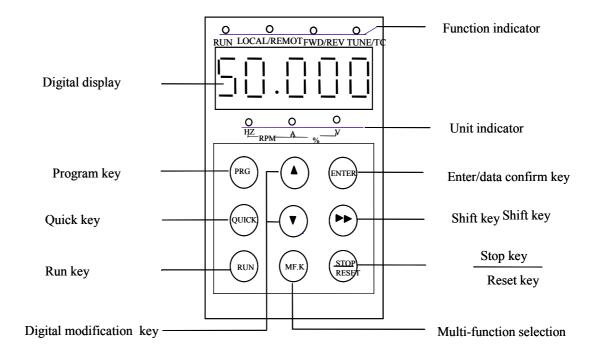
Fig. 4-1 Operation Panel Schematic Diagram
