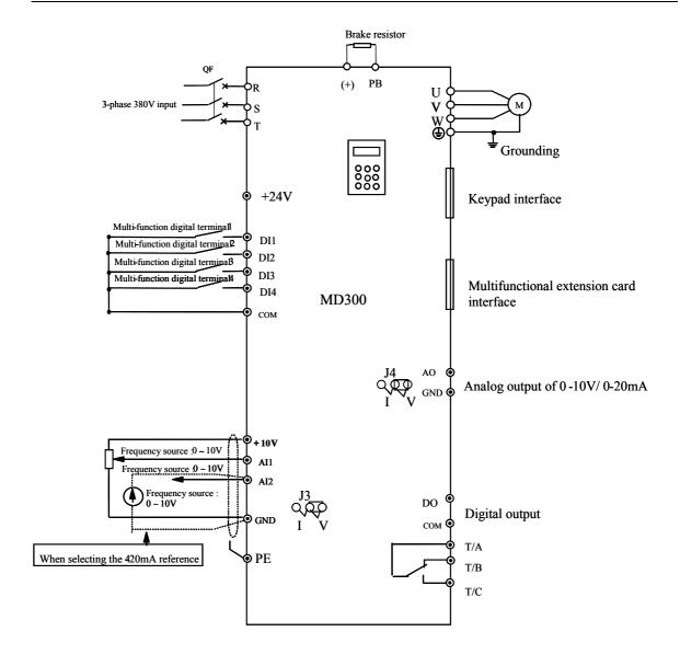
Fig.3-5 Wiring Mode of Three Phase 380V Inverter
