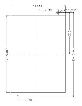
Fig.2-4 Keypad Installation Dimensions
