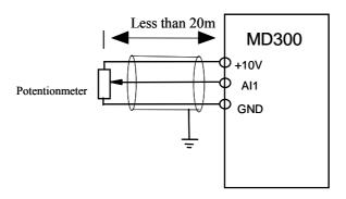
Fig. 3 -6 Analog Input Terminal of MD Series Inverter
