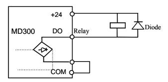
Fig. 3 -8 Digital Input Terminal of MD Series Inverter
