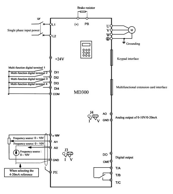
Fig.3-4 Wiring Mode of Single Phase 220V Inverter
