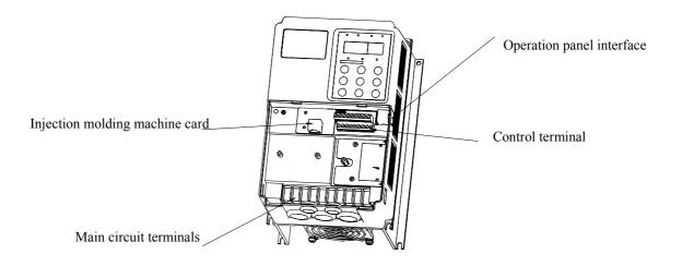
Fig.2-5 Installation of optional parts
