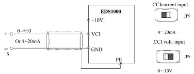
Fig.3-12 CCI terminal wiring diagram
