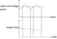
Fig.6-38 overvoltage stall function
