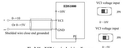
Fig.3-11 VCI terminal wiring diagram
