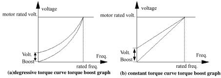
Fig.6-4 torque boost graph
