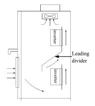
Fig. 3-2 mounting of multiple inverters
