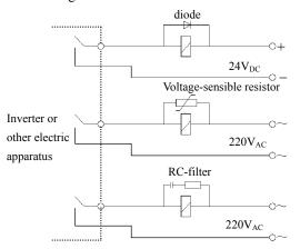
Fig.3-21 installation demand for electromagnetic on-off device
