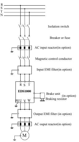
Fig.3-8 connection of inverter and fitting parts
