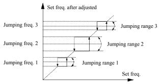
Fig.6-12 jumping frequency and range graph
