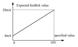
Fig.6-15 specified value and expected feedback value
