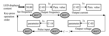
Fig. 4-6 waiting status parameter display operating example
