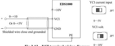
**Fig.3-13** YCI terminal wiring diagram <sup>0</sup>
