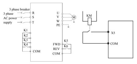
Fig.6-25 multi-step speed run
