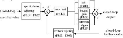
Fig.6-14 PID control principle diagram
