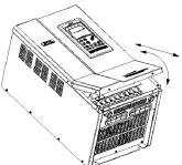
Fig. 3-4 disassembly and mounting sketch of plastic cover
