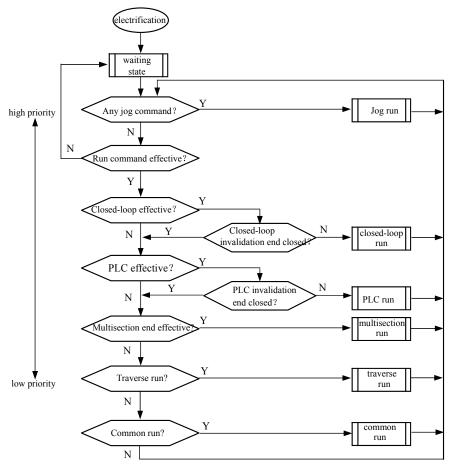
Fig.4-1 logic flow chart of EDS1000 inverter run state
