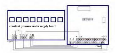
Fig.10-7 connection between water supply controller and inverter
