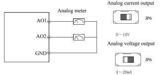
Fig.3-14 analog output terminal wiring
