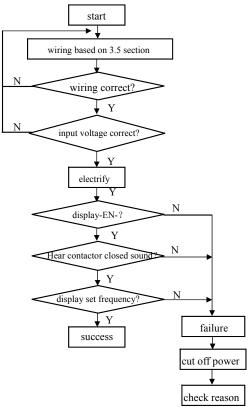
Fig. 4-12 first electrification operation flow
