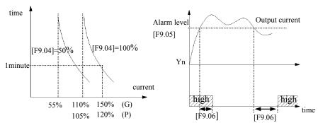
Fig.6-36 electronic thermal relay protection Fig.6-37 overload alarm
