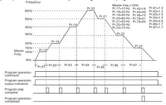
Note: The above diagram shows one complete PLC cycle. To restart the cycle, turn the PLC Program input off and then back on.
