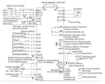
NOTE: Do not plug a Modem or telephone line to the RS-485 communication port, permanent damage may result. Terminal 1& 2 are the power sources for the optional copy keypad and should not be used while using RS-485 communication.
